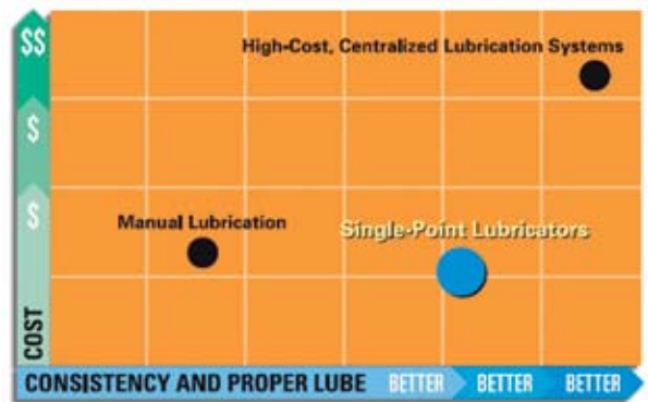
This chart compares the cost vs. effectiveness of different types of lubrication systems.
